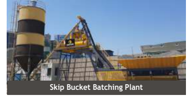
Skip Bucket Batching Plant
